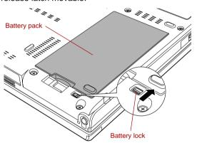
Figure 6-1 Releasing the battery pack (1)
